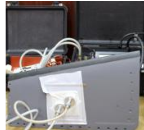
Mounting the heater on the testing composite panel and prepare the vacuum bag
