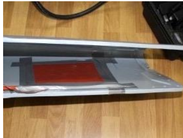
Mounting the heater on the testing composite panel and prepare the vacuum bag
